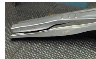
Failure under Stretch-bending (DP780 steel Shown)
