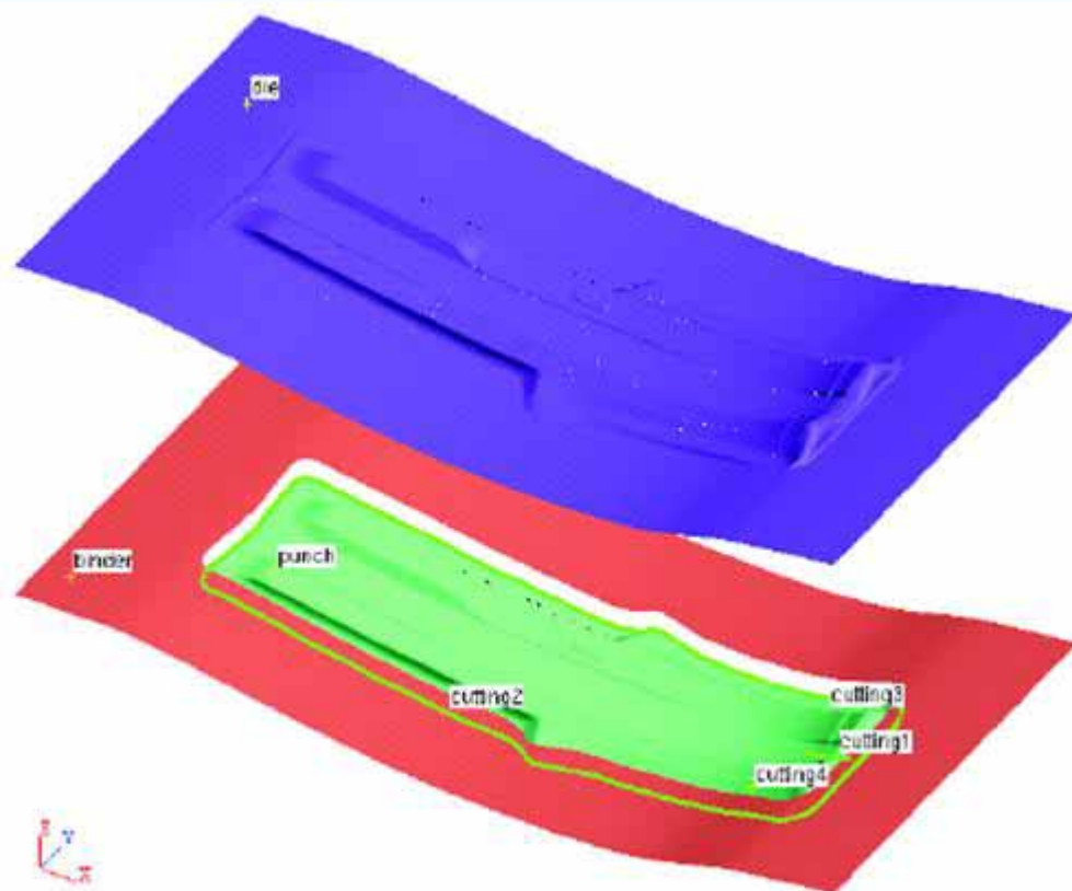
Tool geometry of Lesson 5 with cutting lines
