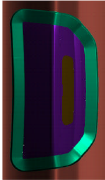
Fig 2.3.2 Profile directions are orientated perpendicular to the part and do not follow the feature-lines
