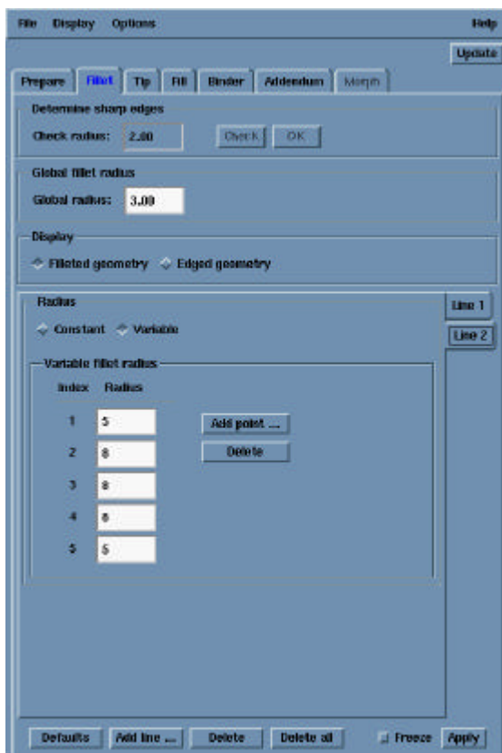
Fig 2.7.3 Definition of an edge with variable radii
